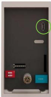
Micro USB connector on the back of the MTPX-MF-SA reader for an easy programming
