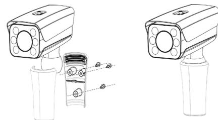
Step 1 Insert the damping ring and waterproof ring of cable into the bracket housing.
