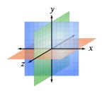
The ANPR engine recognizes license plates in angled positions in all planes. Information about horizontal and vertical angles is covered before. The license plate itself can also be tilted in the x & y axis plane. This angles can be 10° maximum.
