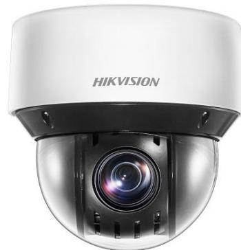
Hikvision DS-2DE4A425IWG1-E 4 MP Network IR PTZ Camera adopts 1/2.8" progressive scan CMOS chip. With the 25 × optical zoom lens, the camera offers more details over expansive areas.
