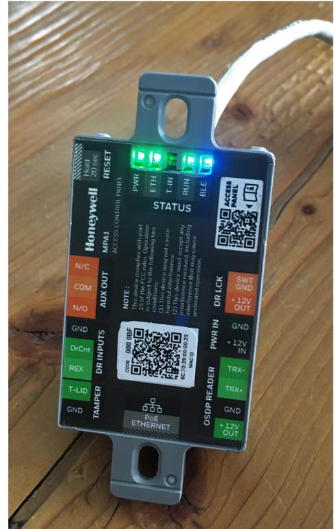
**Note:** If the BLE LED is not blinking on the panel then user need to press the Reset button. The panel reboots and the BLE LED AND RUN LED start blinking. For more issues, see the FAQ section.
