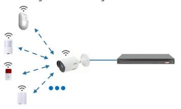
Connect the wireless node devices to XVR with gateway camera and then configure parameters.
