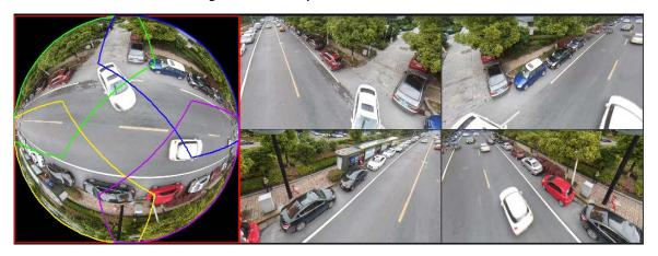
You can use the mouse to drag the color areas on the left original screen or the rectangular screens on the right to change the monitoring ranges. (Not supported for wall mount.)
