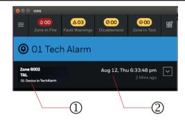
The above example shows a Technical Alarm 'TAL' from a device 1 that occurred at time and date shown 2 and is linked to Control Zone 6002.
