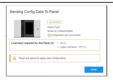
The Tool will display successful transfer of configuration file, if there are Licence required then this will be indicated here, select **DONE** when finished.
