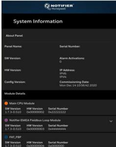
Notice the 'System Information' screen will pop up and show Modules installed in the Panel. Scroll down to the first Loop Module, select the down arrow on the right to view Loops. Notice the device count is initially '0 devices'.
