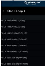
O7 Rectify the displayed faults on the loop. Fault can be filtered and viewed. Upon rectification the fault will clear on the display.
