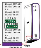
Do not use  $3 \pm 88 \pm .$ Loop cable screen must be connected to the Earth Bar. OS Connect the HMI cable to the CPU module.
